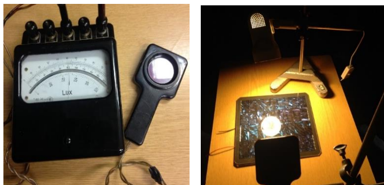
Fig. 1. Lux meter and experimental layout for measuring the reflected light polarization
